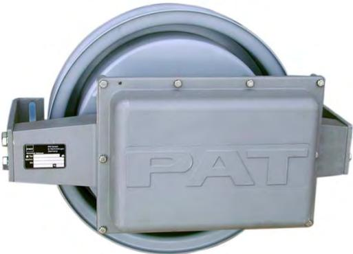
**The Length-Angle Transducer:** The length-angle sensor (LWG), often referred to as the “cable reel”, is a combination of two transducers in one unit. It is installed on the base section of the boom and measures the length and the angle of the boom.
