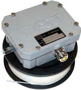
The length sensor (LG105), also known as a “cable reel”, the reeling drum drives a potentiometer, which is the length transducer.
