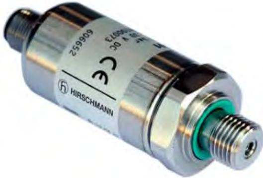
The pressure transducer converts hydraulic pressure into an electric signal. Every pressure transducer has its own CAN Bus converter board, and it has its own device Node-ID. The piston oil pressure transducer is connected to the piston side of the lift cylinder, its Node-ID is 0x3C; The rod oil pressure transducer is connected to the rod side of the lift cylinder, its Node-ID is 0x3D.
