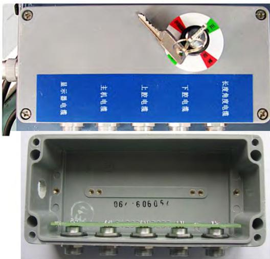
The CAN Bus junction box contains a CAN patch board with five sockets which can be connected with five different CAN nodes.
