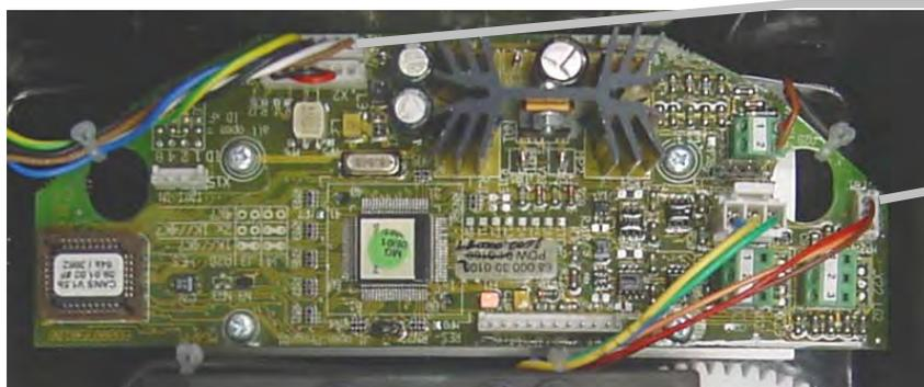
*CAN Bus electronics in cable reel.*
